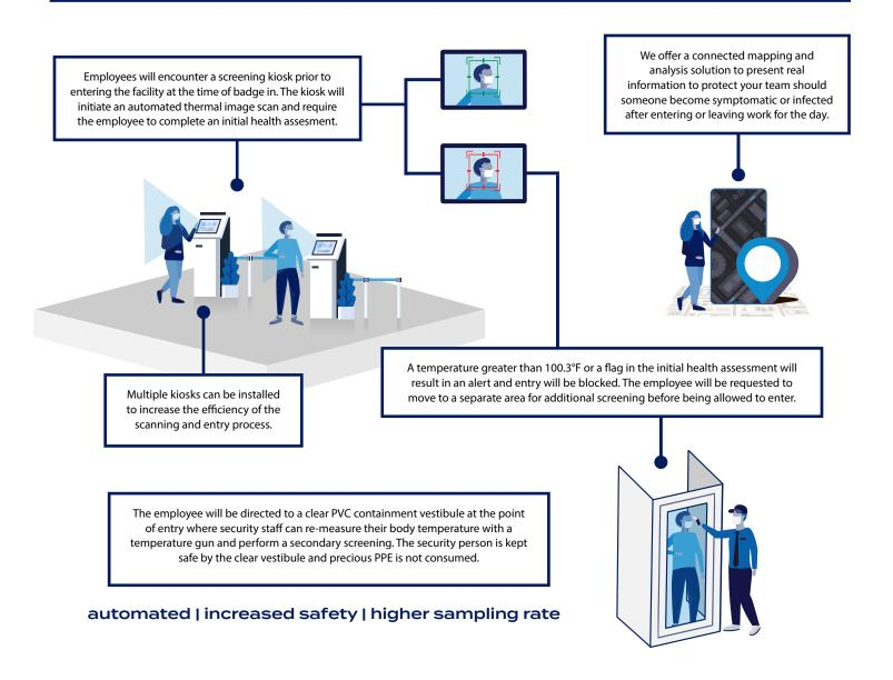
To avoid HIPPA concerns, the thermal image scan triggers a "latching relay" response to allow entry in conjunction with the security badge scan already in place. The thermal image and body temperature is not attached to the person's identity. The information is not saved and therefore cannot be disseminated beyond the go/no-go entry decision at the badging location.
